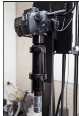
Queensland Museum's upgraded Visionary Digital BK-Plus imaging system. L. to R. 1. Overview. 2. Canon 5DS with Canon MP-E 65mm 1:2.8 1-5x macro lens. 3. Canon 7D MkII with Dun Inc. microscope and 10X Mitutoyo microscope objective.
