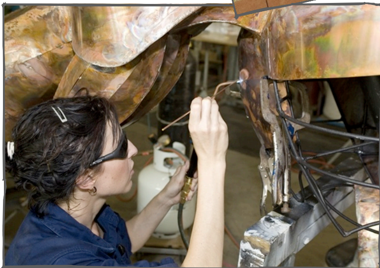
Fig.3. The artist oxy-welding formed copper plates on to the steel framework of the head of the 7.5 metres ant. Above her head is the completed fore coxa and prothorax.
