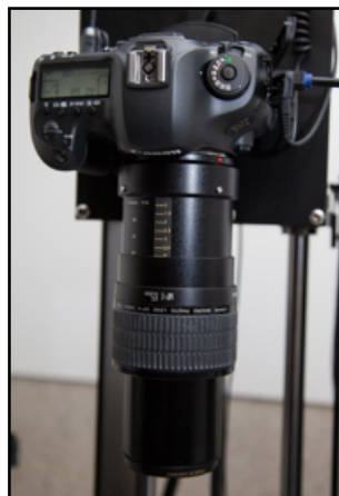
Queensland Museum's upgraded Visionary Digital BK-Plus imaging system. L. to R. 1. Overview. 2. Canon 5DS with Canon MP-E 65mm 1:2.8 1-5x macro lens. 3. Canon 7D MkII with Dun Inc. microscope and 10X Mitutoyo microscope objective.
